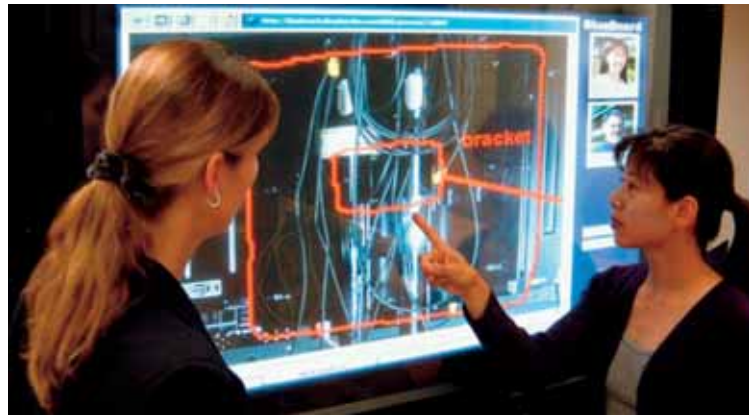
5 BlueBoard provides a digital whiteboard for freehand drawing and writing, a Web browser, and access to personal data repositories.
