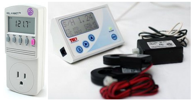
Figure 1. (left) The Kill-A-Watt plug-in load meter. (right) The Energy Detective uses sensors that clip-on to the home's main circuit breaker.
